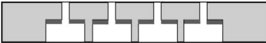
Fig. 7b Typical cross-sectional view of the top-layer structure showing cavity, electrode, and channels for each actuator.
